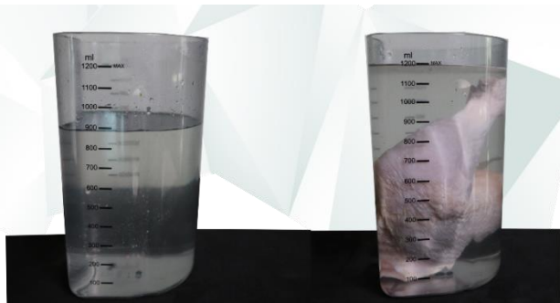
Determining the volume of an object based on changes in the height of the liquid column
