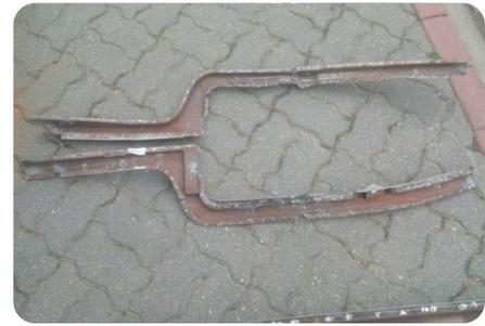
**Fig. 2.** Measured object: corroded pillar B removed from a T1 Transporter.
