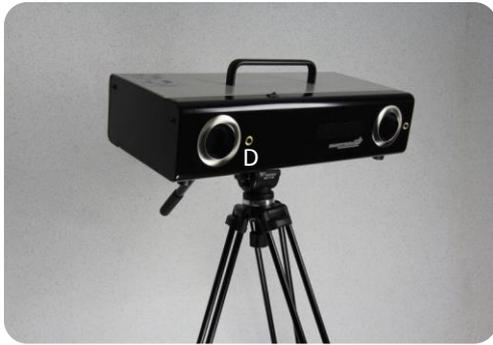
*Fig. 4. Optical measurement system scan3D surface.*
