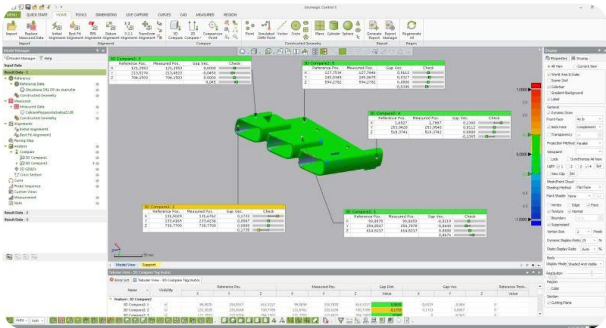
Fig. 5. Optical inspection result in Geomagic Control.
