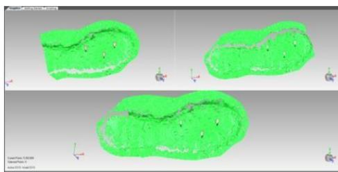
Preliminary scan alignment using the 3-point method
