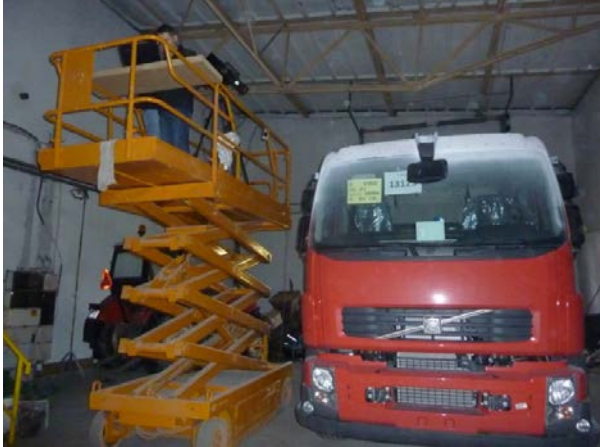
Scanning process – 3D scanner placed on a lift
