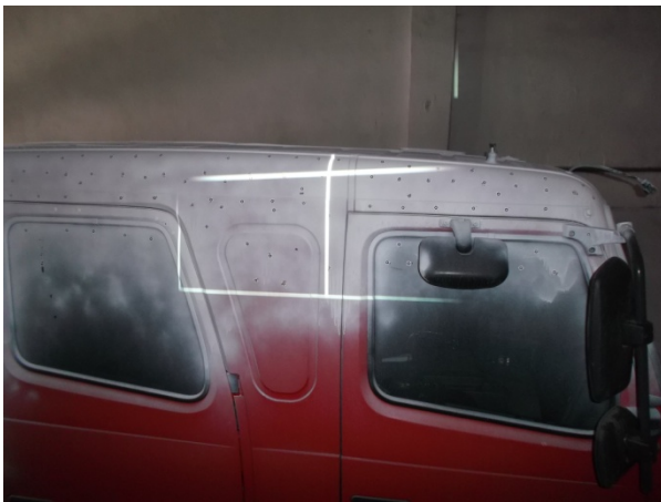
Surface of the vehicle covered with a matting solution with attached reference markers
