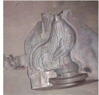
At the request of his client, the glassworks Edwanex manufactured 500 pieces of occasional glass bottles which design was not used in the bottling plant for over 20 years. The unusual shape of a rooster was supposed to be achieved on the basis of an old mould that was unsuitable for use due to corrosion and nicks. By using the 3D scanner from SMARTTECH it was possible to quickly recreate the original, unique shape.
