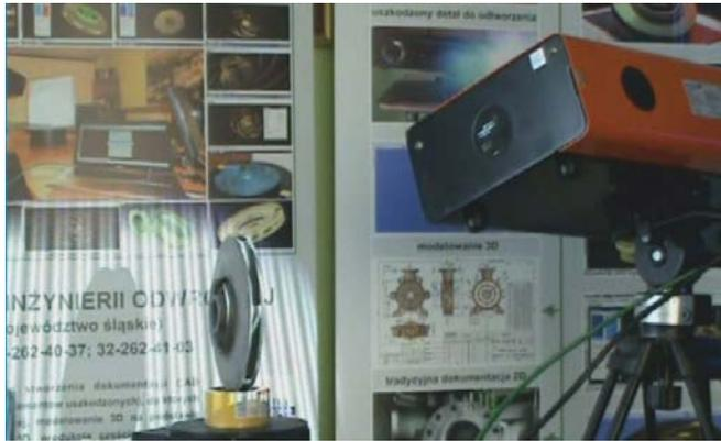
Having SMARTTECH 3D scanner scan3D surface 5Mpix - Ekoglob is able to receive 5 millions of points that describes measured surface within few seconds and with the accuracy of 60 microns. Scanner field of view is 600x400 mm, however they are not limited to this size, thanks to possibility of connecting single scans automatically using positioning markers. By sticking markers to the object we practically divide the surface to parts, that
