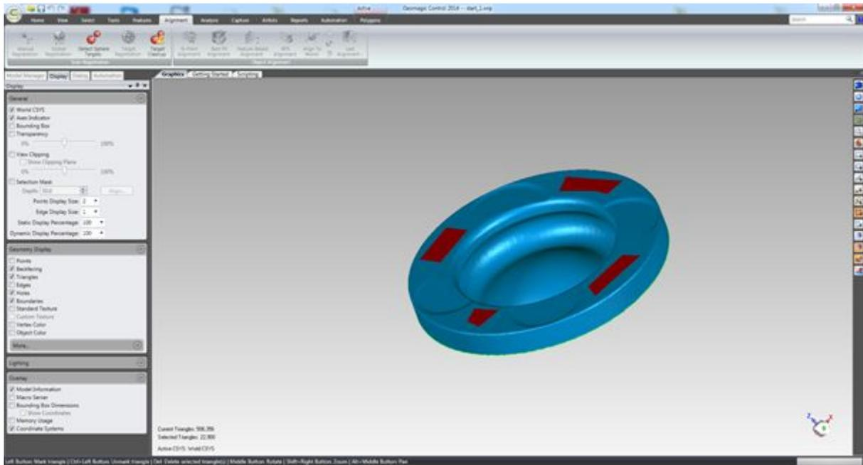
Fig. 5.1 Areas used to create a reference plane.
