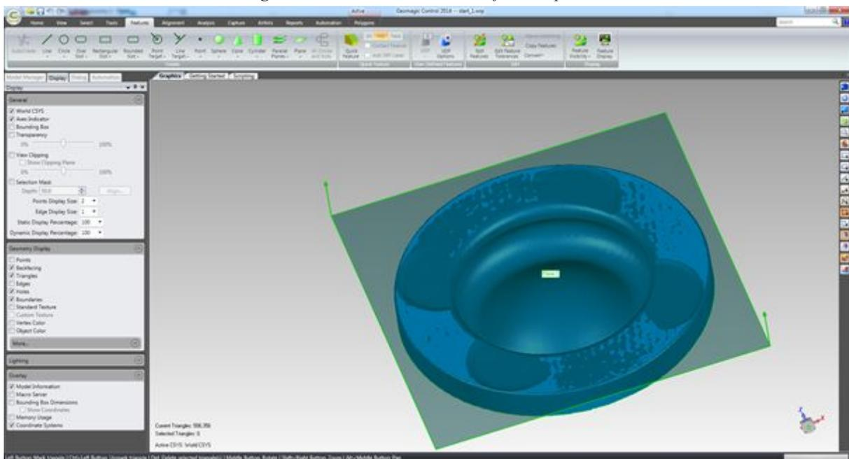
Fig 5.2 Areas, a reference plane, to which a piston volume was calculated.
