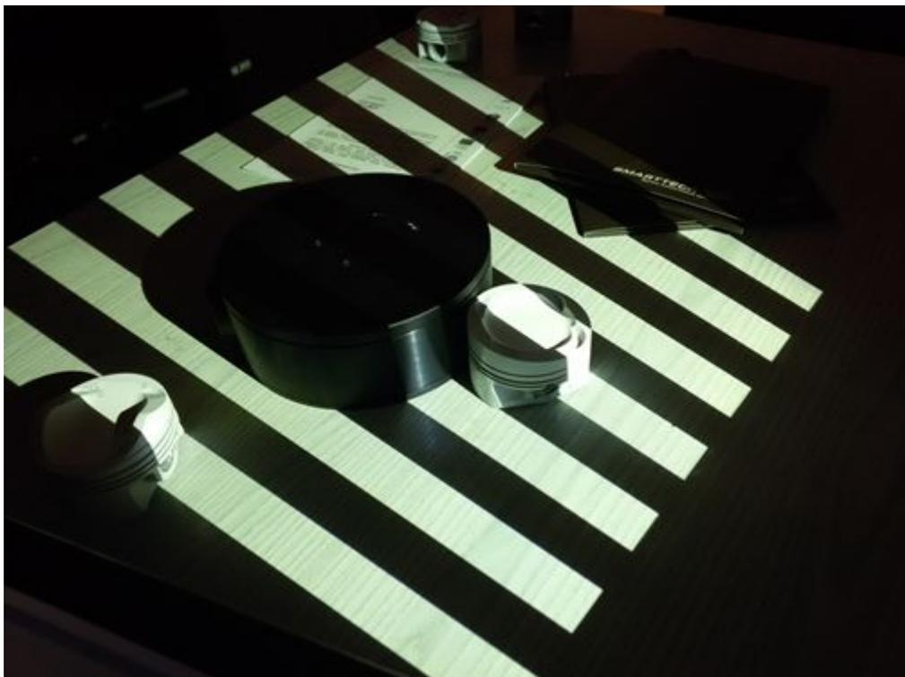
*Figure 2.1 The scanning process*
