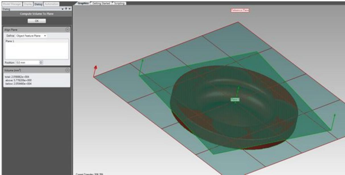
Fig. 5.3 Areas used for the creation of the reference plane..
