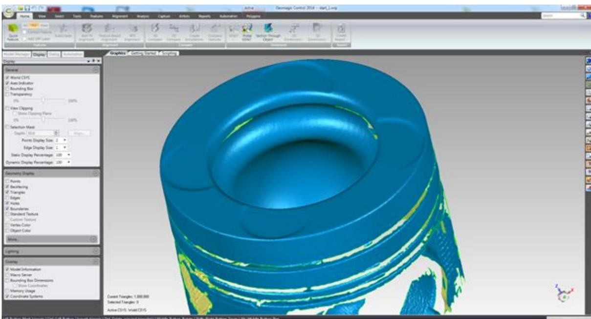
*Fig. 4.4 Triangle mesh in Geomagic Control*
