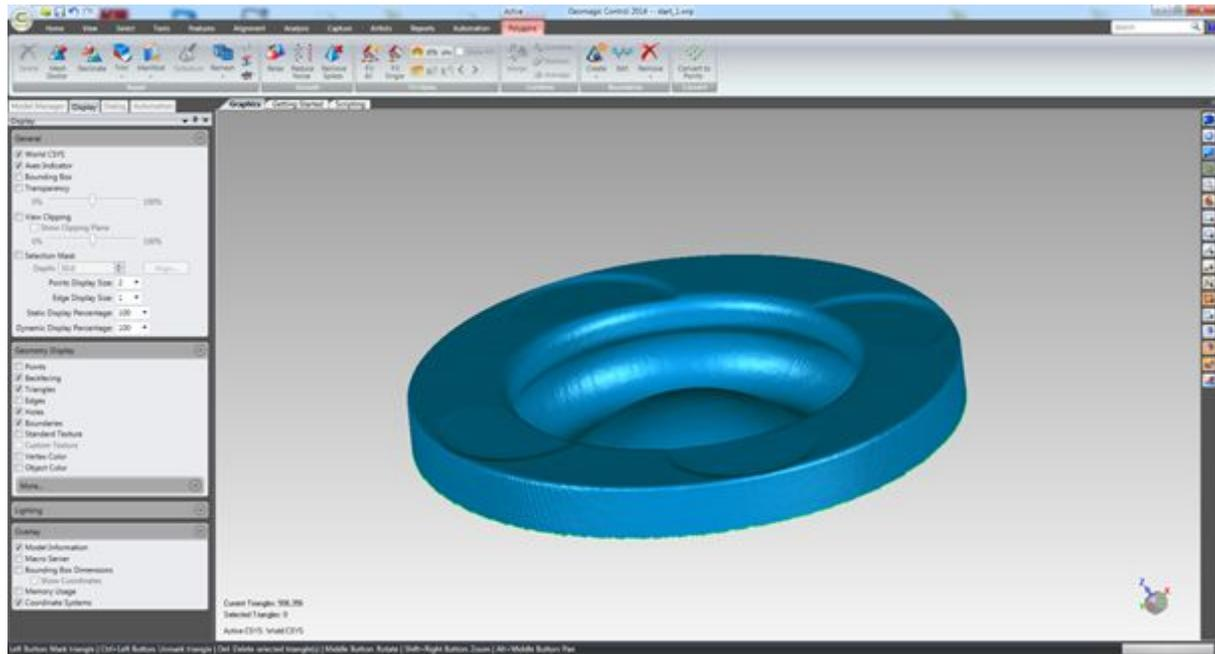
*Fig 4.5 Prepared triangle mesh in Geomagic Control.*
