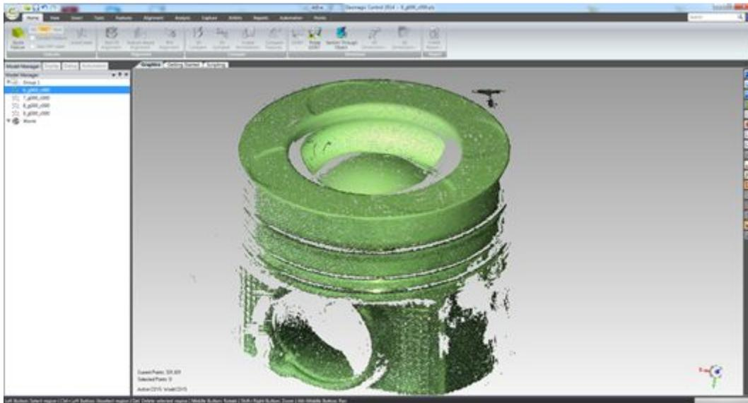
*Fig. 4.1 View of the point clouds in Geomagic Control.*
