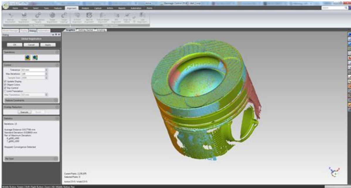
*Fig. 4.3 Accurate aligning in Geomagic Control.*
