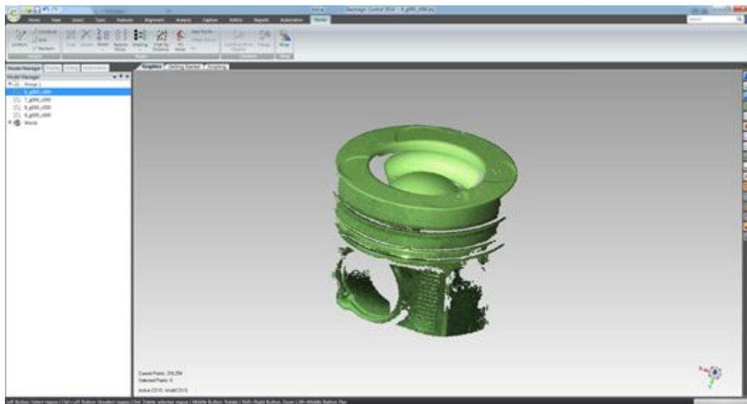
*Fig. 4.2 View after the noise cleaning in Geomagic Control*
