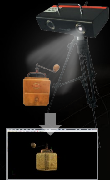
Raw scanned data - cloud of points with texture (XYZ,RGB)
