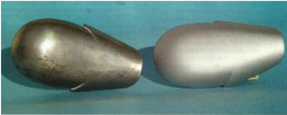
*Replica part (left) and 3D printed pattern (right)*
